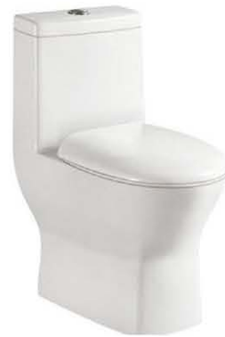
WCC 108 Siphonic One-Piece Toilet Size: 620X360X710mm S-trap, 300mm Roughing-in
