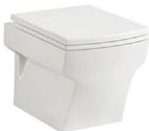
WCC 307 Washdown wall-hung Toilet Size: 485X340X350mm P-trap 180mm Roughing-in
