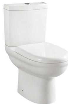
WCC 203 Washdown Two-Piece Toilet Size: 610X400X790mm P-trap 180mm Roughing-in
