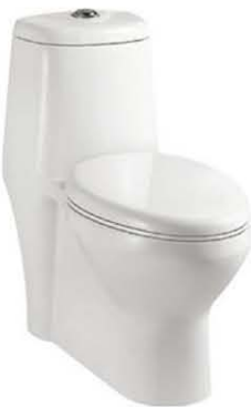
WCC 107 Siphonic One-Piece Toilet Size: 730X390X750mm S-trap, 300mm Roughing-in
