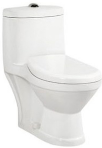
WCC 113 Children's Washdown One-Piece Toilet Size: 520X280X530mm S-trap 180mm Roughing-in
